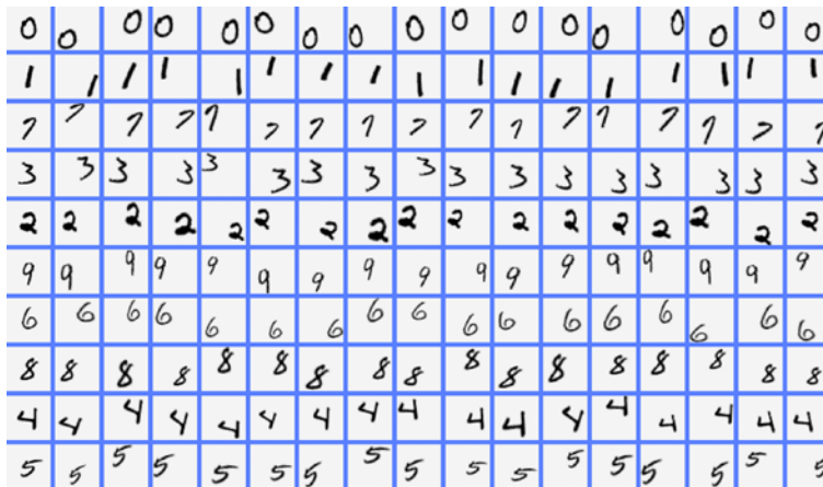
Figure D.3 The entries in the leftmost column are examples from the original MNIST; the other columns are all affine transformations of the data included in affNIST [image credit: “affNIST” ( http://www.cs.toronto.edu/~tijmen/affNIST )].
